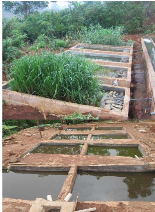
Vegetated beds and Lagoon systems for wastewater treatment experiments
